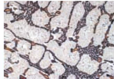
Microstructure: ferritic matrix containing primary and secondary carbides
