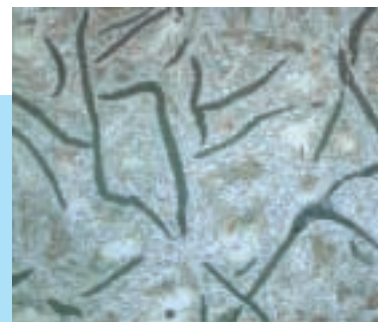
Microstructure: bainitic matrix containing lamellar graphite
