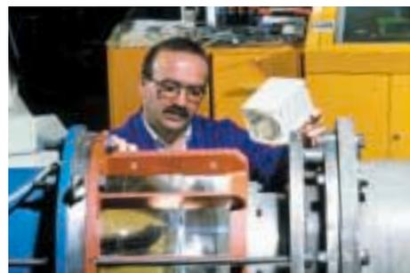
*Feed pumps being tested under operating conditions on KSB's own test rigs (top photo)*
