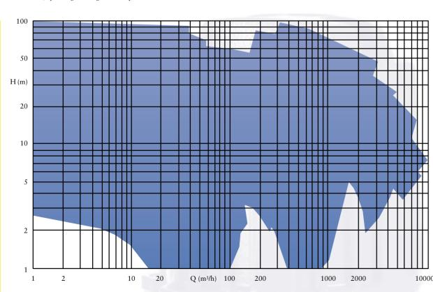
KSB-Know how: The use of different impeller types is the means to optimise performance data with regard to the pumped medium
