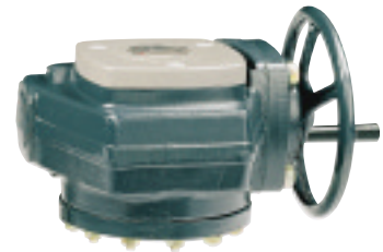
M31 - Variable torque advantage output for reduced input force, cast iron housing, bronze and steel internals, roller bearings, direct mount limit switch capability, visual indication, epoxy coated.
